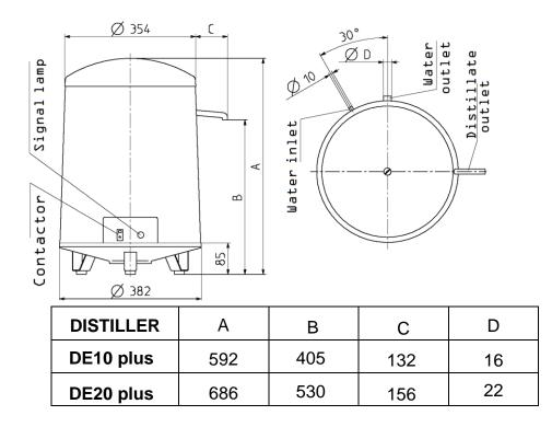
Fig. 1 Distillers external dimensions
